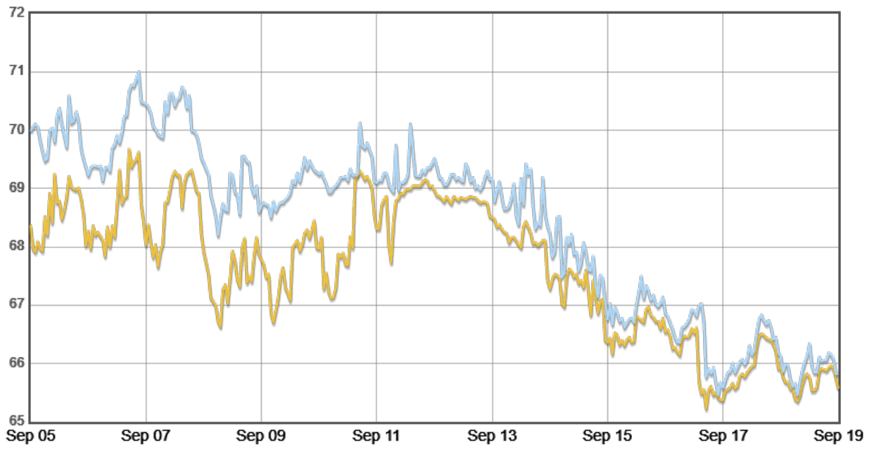
Figure 1. Lower Granite fish ladder exit pool (blue) and forebay (yellow) temperatures September 5-19.
